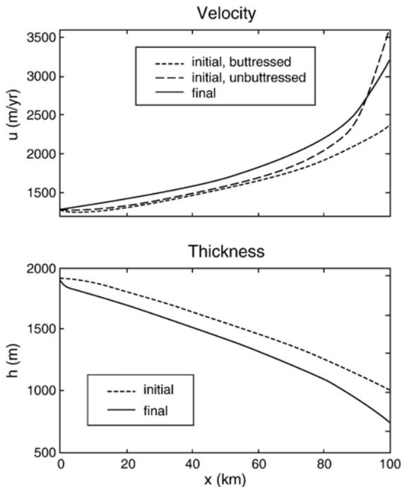
Fig. 5. Effect of ice shelf buttressing on velocity of grounded ice. Removal of ice-shelf buttressing causes ice-flow speed-up and thinning, as described in the text [32].
